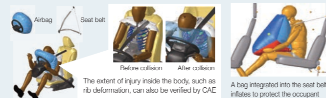
Figure 2: Development of airbag and seat belt set (CAE) Figure 3. Lap airbag
