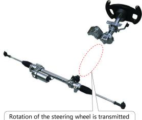
Rotation of the steering wheel is transmitted to the wheels via electric signals. (No mechanical link.)
