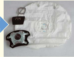
Dismantled airbag for recycling
