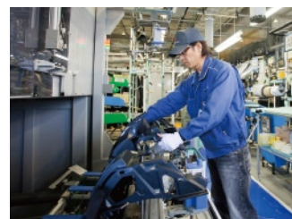
Movable jig with a shifting switch
