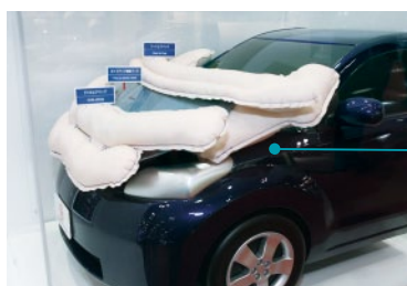
Pedestrian protection airbags (under development) Airbags that inflate in the event of a front-end impact to protect pedestrians
