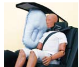
Backseat Center Airbag Airbag due to protect passengers in sitting opposite side from collisions
