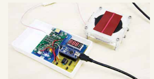
Reproducing the beating of the heart by taking advantage of the characteristics of e-Rubber, which maintains its properties well and moves quickly
