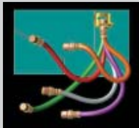
Brake hose routing simulation
