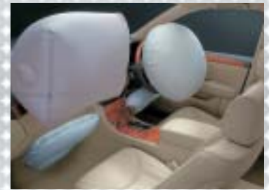
Dual-stage driver- and passenger-side airbags and knee airbags (above) Side airbag and curtain airbag (left)
