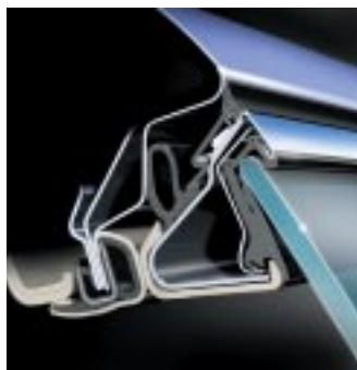
Stress distribution analysis (above) Cross-sectional diagram of body sealing products for frame door (left)
