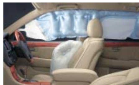
Dual-stage driver- and passenger-side airbags and knee airbags (above) and side airbag and curtain airbag
