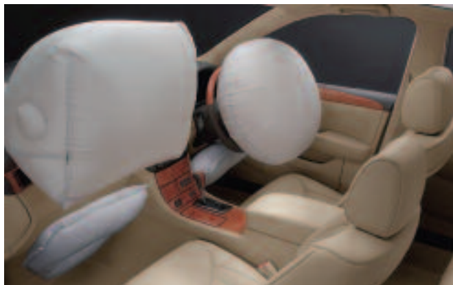
Airbags for up to 10 positions in the vehicle interior to protect the occupants.
