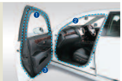
① Glass run ② Opening trim weatherstrip ③ Door weatherstrip that, in combination, provide optimum sealing for any kind of door functionality and design.
