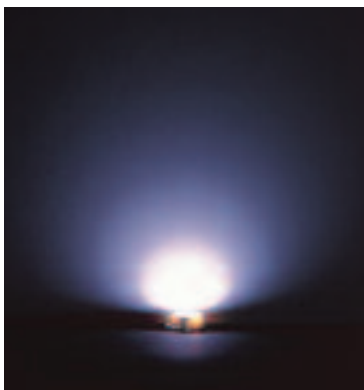
High-luminosity white LEDs suitable for backlights in liquid-crystal displays for televisions and laptop computers and even for future applications in general illumination.
