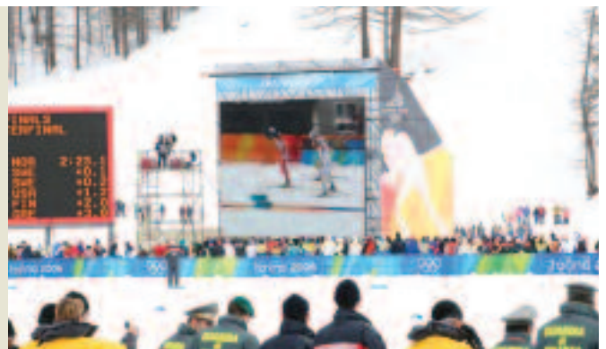
Outdoor LED displays with a wide viewing angle and high visibility, developed for large-scale applications, such as sports stadiums.
