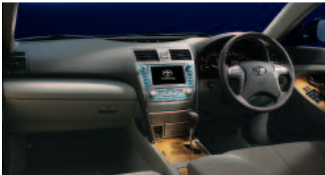
Instrument panel modules that reduce costs and simplify installation by integrating formerly separate components.
