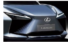
2023 Millimeter wave compatible emblem that emits light
