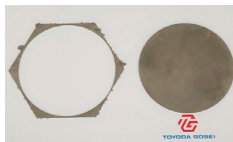
6-inch seed crystal produced from hexagonal Na-flux GaN crystal
