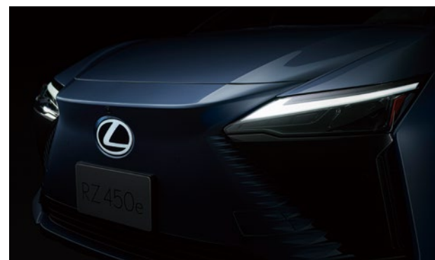
Millimeter wave radar-compatible emblem that emits light
