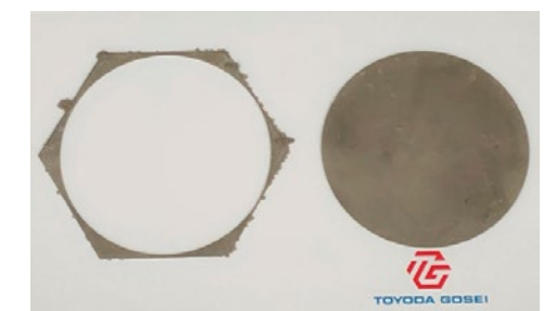
6-inch seed crystal produced from hexagonal Na-flux GaN crystal
