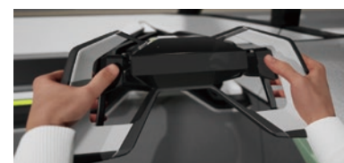
Biometric-sensing steering wheel (such as to detect alcohol)
