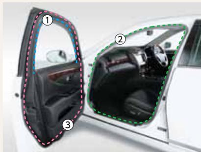
The best door sealing structures are proposed for diverse door function and design needs
