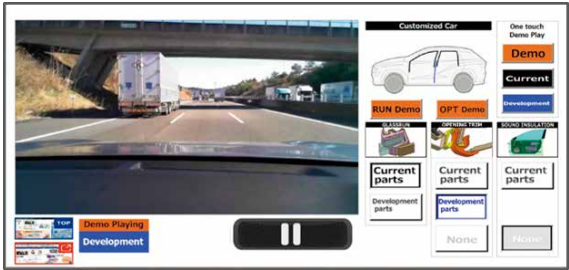
Simulation system to experience the driving sounds that will occur when equipped in vehicles.
