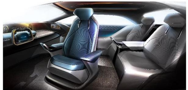
Airbags are integrated into seats to accommodate the more diverse occupant postures that are expected with autonomous driving.
